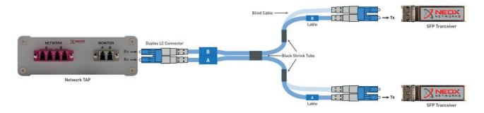
This image shows a Y-cable that NEOX offers to complement its passive (modular or portable) Fiber TAPs. As you can see the Y-cable is designed in such a way that the light from the TAP (which is connected on the left side of the above diagram) is correctly directed to the two receive ports of the transceivers (which would be on the right side).
