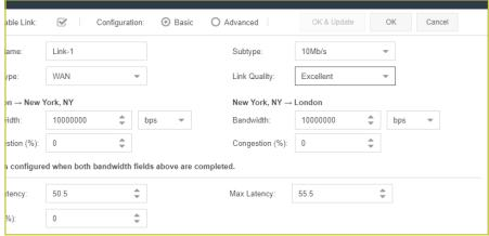
Define two endpoint locations, set the link type and quality. Default Latency and Loss values will be automatically calculated which can be customized if required.
