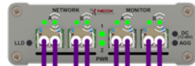
Link and traffic present on all ports; the left LED lights up continuously and the right LED flashes.
