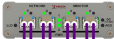
Link present on all ports; Left LED lights up permanently in each case
