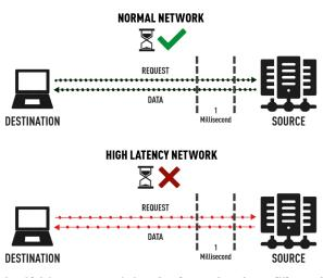
In a high latency network, less data is transferred per millisecond Figure 3: Difference between normal and high latency. Each point in the network traffic illustrated above represents an Ethernet frame!
