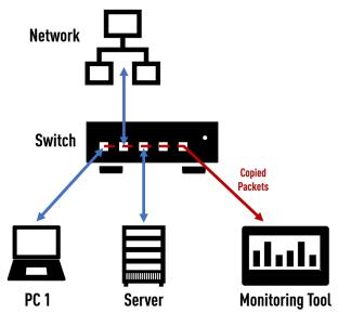
Figure 1: Functionality of a SPAN/Mirror port
